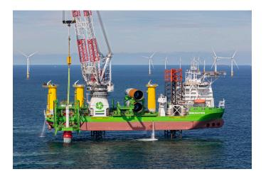
overall gripper weight down. The unique combination of gripper stiffness with the slenderness of the construction enabled DEME to maximize the useful payload on its jack-up. Our unique Pendulum Design increased the versatility and pilling accuracy of HLJV Innovation.
