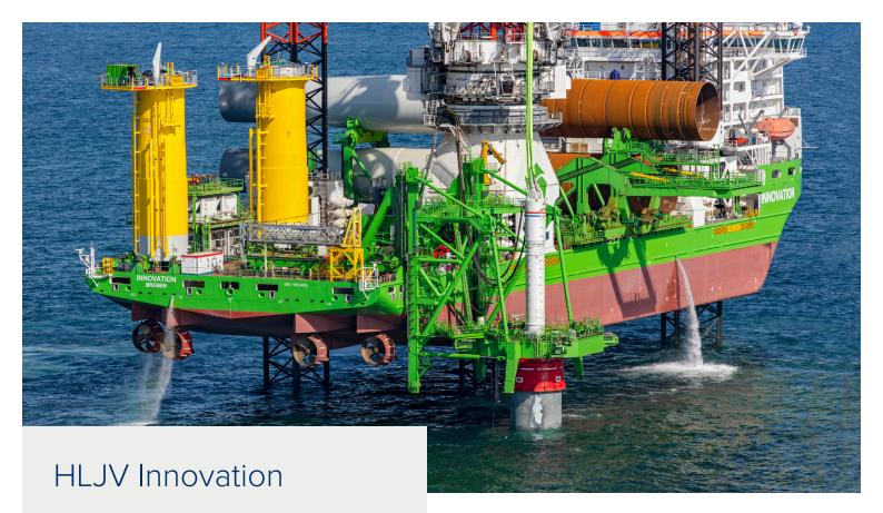
The Heavy Lift Jack-up Vessel [HLJV] Innovation is a dedicated offshore wind vessel from DEME that installs monopile foundations. To scale up the monopile installation capability of HLJV Innovation, DEME came to TWD with requests to design a tailored monopile gripper and the related installation equipment.
