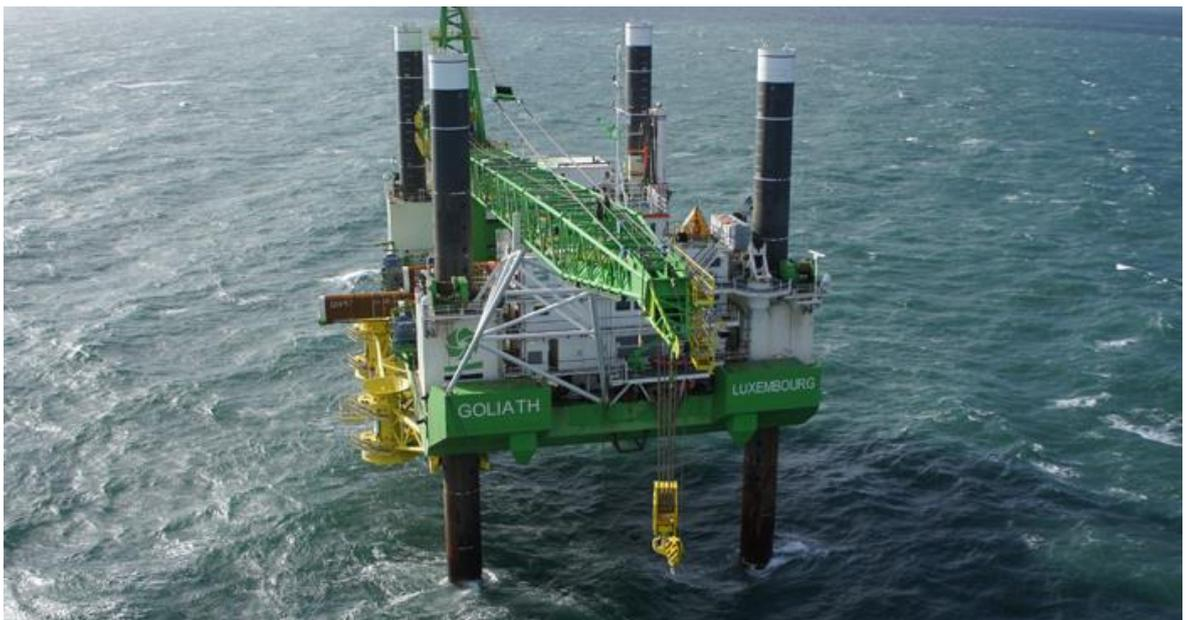
*Jack-up barge with TWD designed piling template for installation of wind turbine foundations*
