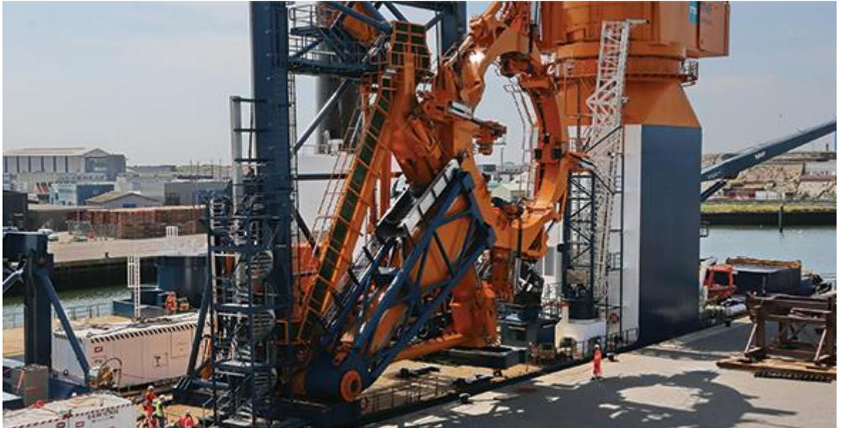
*Monopile gripper frame onboard of the Aeolus*
